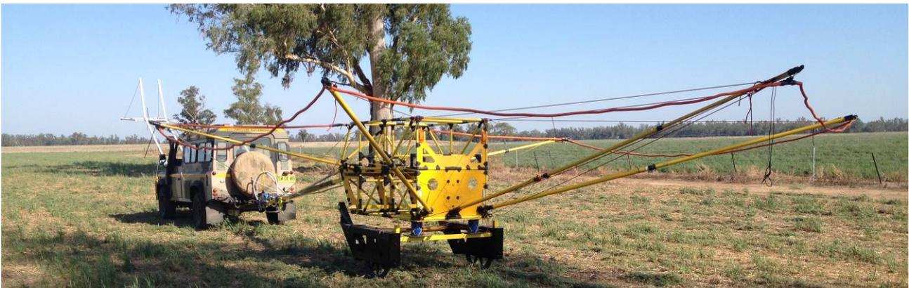
**Figure 1: AgTEM<sub>4</sub><sup>TM</sup> cart with an additional receiver loop forward of the towing vehicle.**
