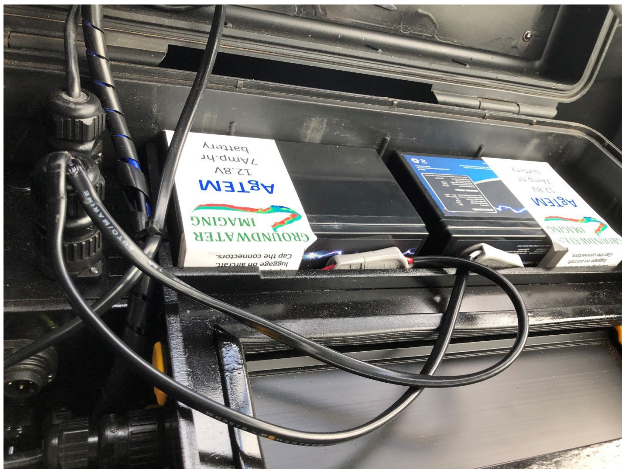
Figure 42 Battery space in the receiver accessories case houses either two 7AmpHr or two 12AmpHr 12.8V batteries even when the case is fully packed and closed. More can be housed and connected while the case is open in operating mode or if the display housing lid is swapped to another case.
