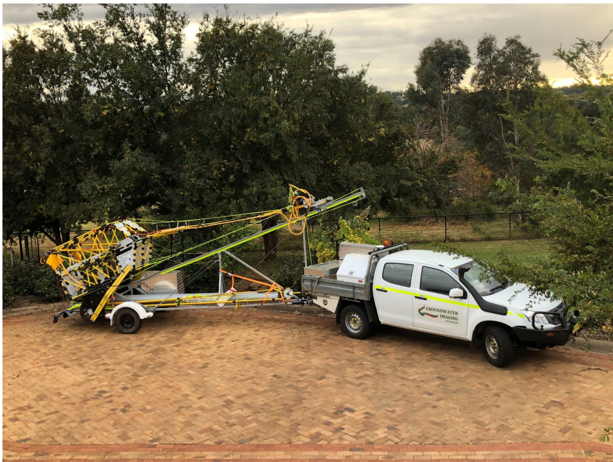
Figure 19 The quick deployment float trailer. The Wallaby is shown at 4.5m drawbar length but the trailer can also accommodate it set at 5m drawbar length.
