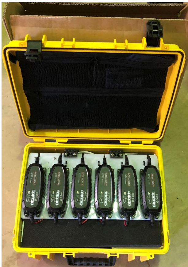
Figure 38 7AmpHr battery charger and housing box. Leaving this in the towing vehicle with batteries inside is an efficient way to operate - providing loop and electronics power to the transmitter but 60AmpHr 25.6V batteries will be better should you not need to airfreight. As of January 2025 these have been replaced with Victron chargers as the type shown cannot restart the BMS on LiFePO4 batteries if the battery triggers the low voltage cutoff.
