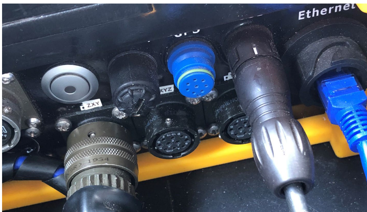
Figure 48 Receiver connections. Single or three component receiver cables may be connected to three different connectors however the components are rotated around successively in each connector such that Z is component 1 in the first, X in the second, and Y in third. Typically the Wallaby receiver loop will attach to the first connector (ZXY) and the front loop will attach to the second connector (XYZ). Note that the blue GPS connector is not currently in use.
