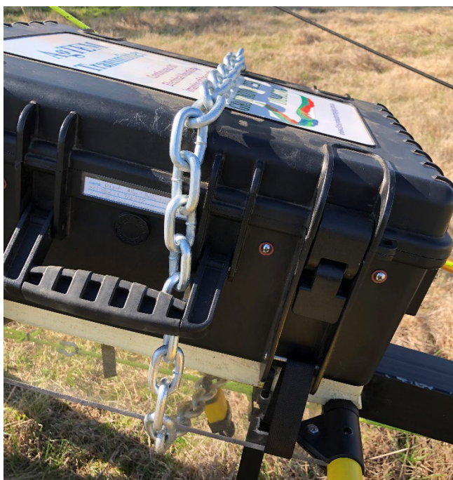
Figure 30 Chain restraint of the transmitter overnight to prevent theft - remove the chain before surveying. As of January 2025 this location for the transmitter is rarely used – preferring to locate it on the towing vehicle to make daily setup and pickup quicker.
