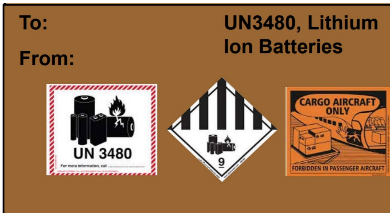
Figure 67 A sample of Lithium Iron Phosphate Battery packaging for commercial freight. Avoid the trouble of this packaging if possible by using <99Whr batteries carried on board aircraft as luggage instead. The above labels are used with dangerous goods declaration 3480 PI 965 IB and either MSDs or 'Lithium battery test summaries'. If carried as luggage all this paperwork and related fees can be avoided.
