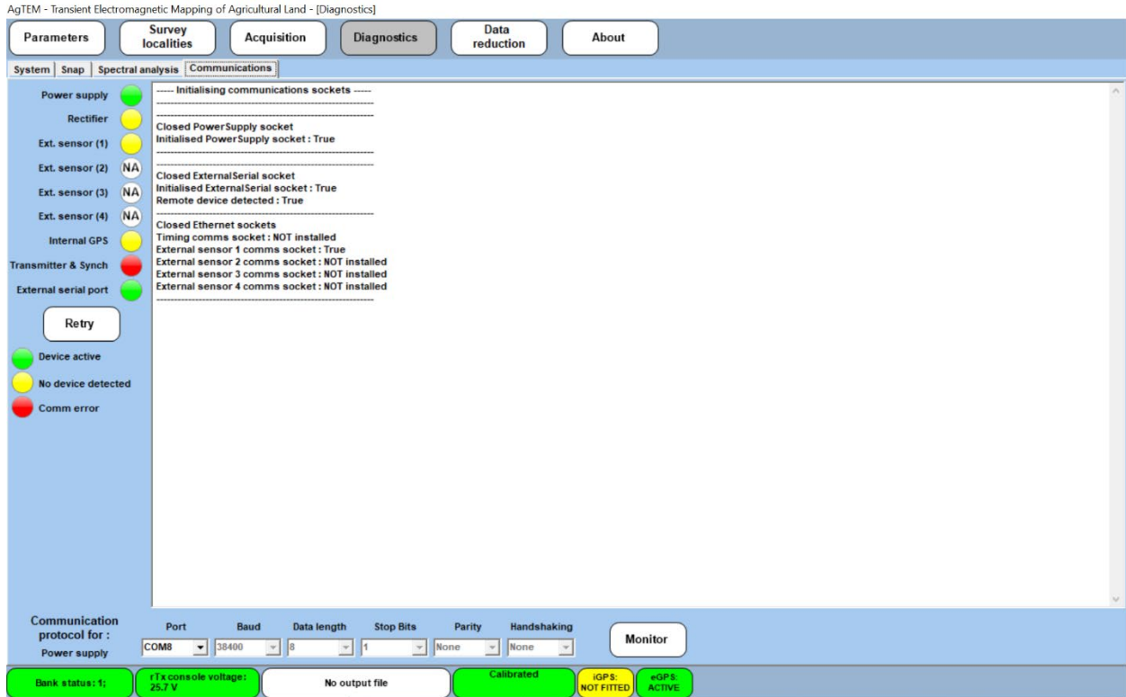
Figure 114 The Communications display after running a communications check by pressing the 'Retry' button.
