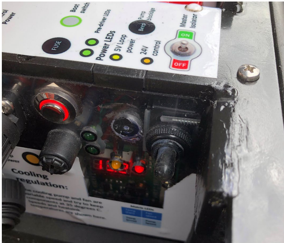
Figure 50 Illuminated transmitter boot button and master isolator switch. If both loop power and control power are connected then both Orange and Red LEDs will light when master power is turned on. Below them cooling performance is displayed but this must be observed from a lower viewing angle than in this photo.
