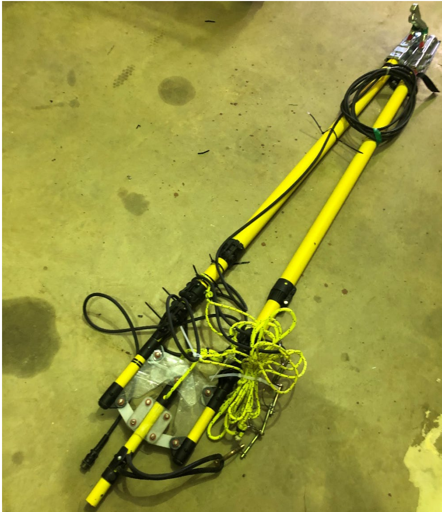
Figure 31 The front loop booms assembly collapsed for freighting.
