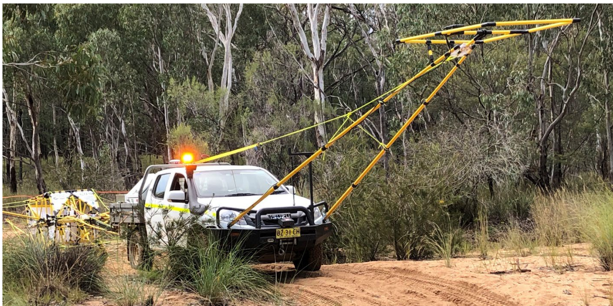
Figure 35 The front loop mounted on tow balls mounted on an Isuzu D-Max bullbar.
