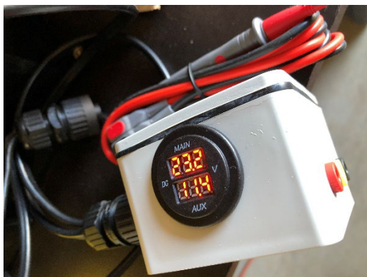
Figure 51 A small stand-alone volt meter that can connect to any battery prior to use to check it is OK and charged. LiFePO4 BMS may switch one of a pair of batteries off altogether while the other still has charge – the dual display will indicate whether both batteries are still OK to use without recharging. Each of the pair is charged individually so balancing problems do not develop.
