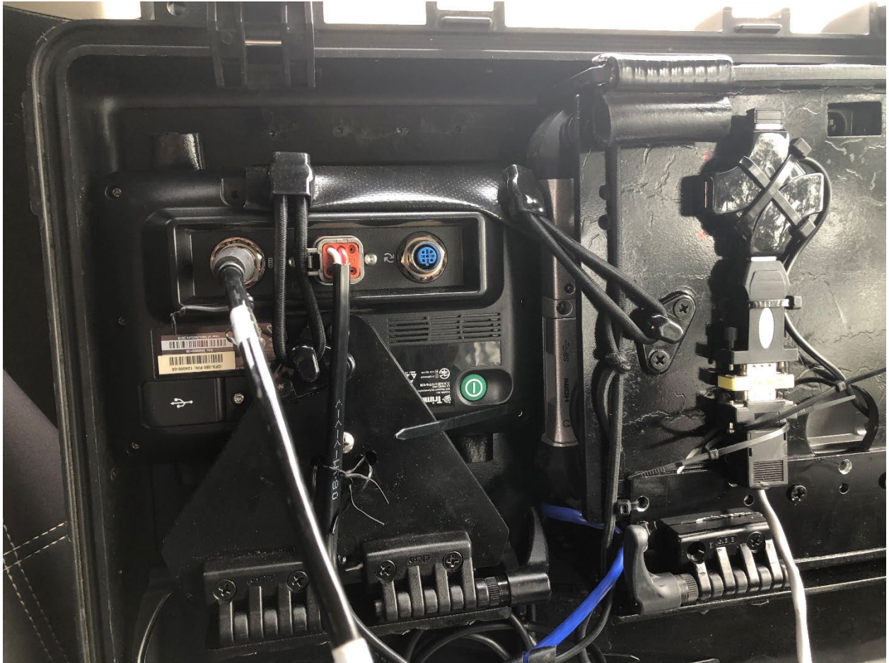
Figure 41 Displays packed within the outer receiver accessories case - detach elastic cords and hinge at double friction hinges to set up for display or remove them altogether for dashboard mounting. This lid housing is provided mainly as a stop-gap measure for temporary installations and freighting – dashboard mounting is the preferred and intended mode of operation of these displays for Wallaby survey.
