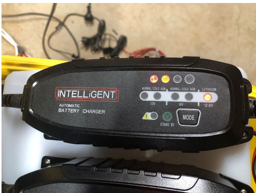
Figure 18 7AmpHr 12.8V battery charger. The Charger is not working correctly unless the Mode mutton has been long-pressed to get the Lithium light to illuminate, and the charge percentage lights in a row at the top have started to illuminate.
