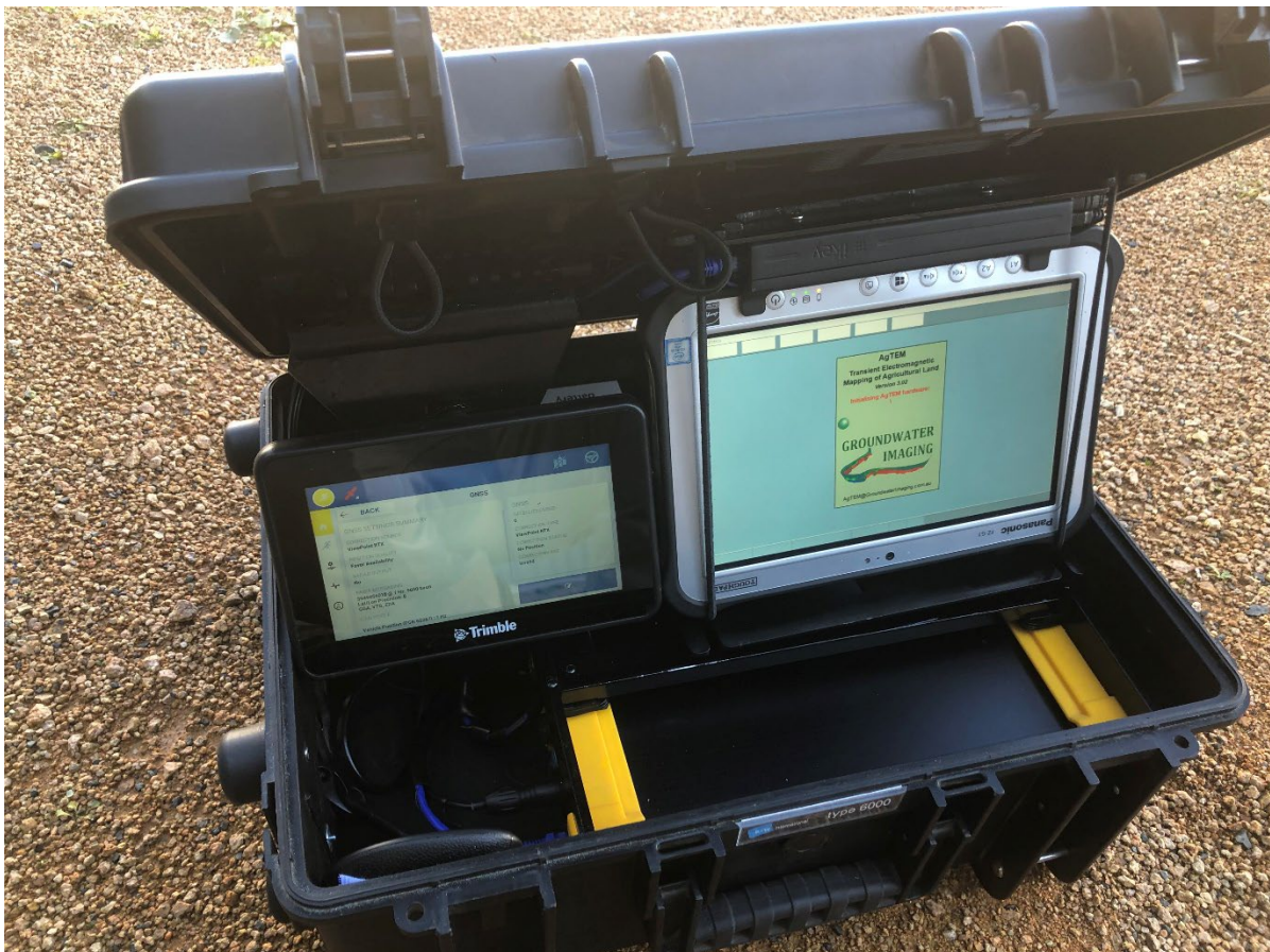
Figure 40 The AgTEM receiver in an outer case with batteries, protected cable connections, external ventilation, Toughpad computer and Trimble GPS display.
