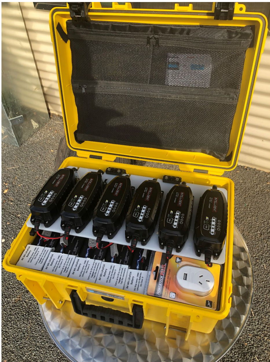
Figure 16 A bank of battery chargers and batteries designed for meeting air carriage restrictions.
