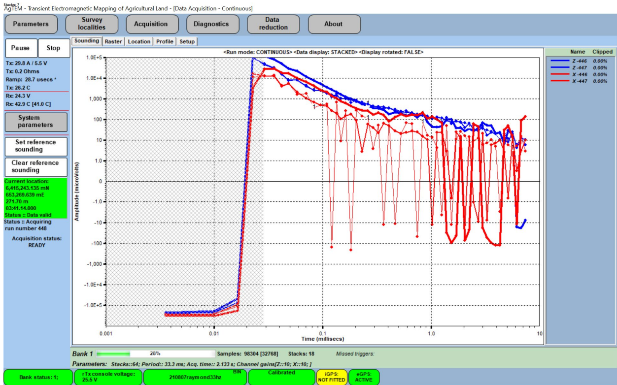
Figure 109 Reference soundings displayed on continuously acquiring 2 channel data with one repeat also showing for each channel. A log-log display has the zero crossing highly amplified so that noise level can be carefully and easily observed. Observe that front loop data shown in red mimics in-loop data at later times – in this case also at early times but that is co-incident in this instance. The grey hashed area displays the ramp time which in this case is measured erroneously large.
