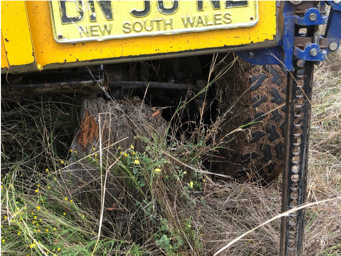
Figure 148 A great example of what you WILL hit if you drive in long grass. This hidden stump was hit in 2nd gear low range. It cost US$700 to repair the steering arm and bash bar damage. It hung up the vehicle – this photo is after winching and reversing.
