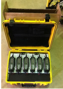
Figure 136 AgTEM battery and charger shipment - note the chargers fold up into the lid and the batteries are in the base of the case. The plastic case is placed in the cardboard box behind for shipping.
