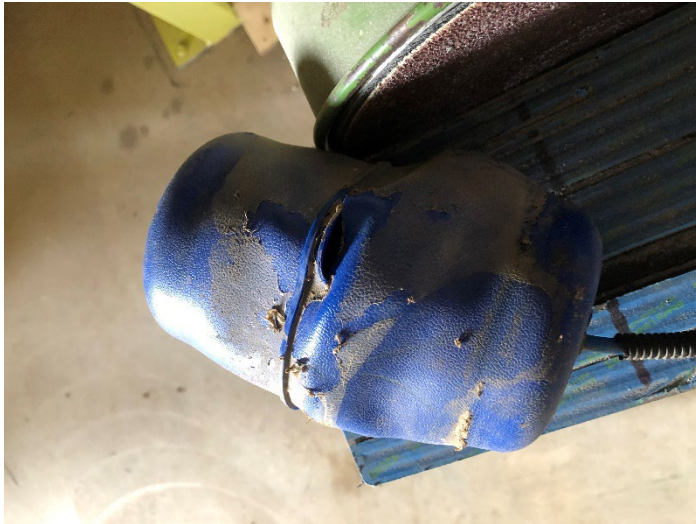
Figure 149 An airbag that burst after being left crumpled at low pressure.
