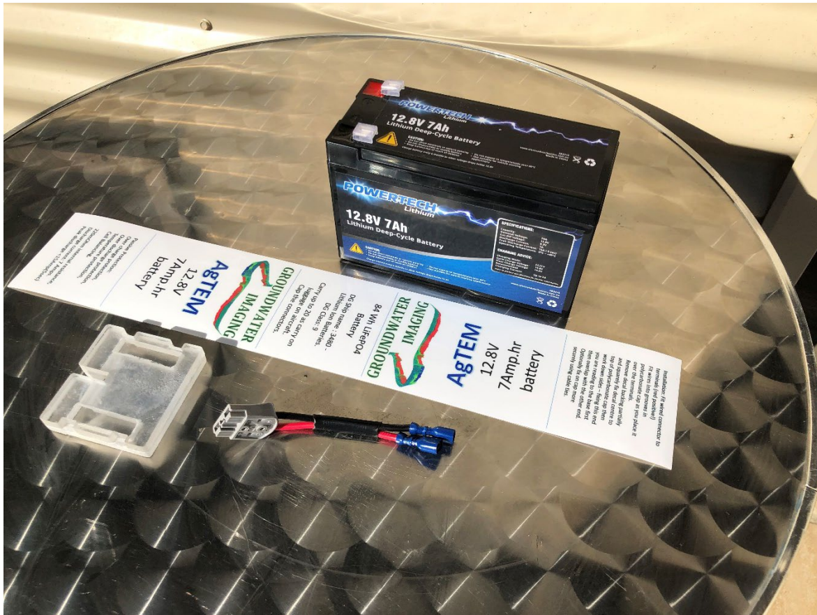
Figure 13 Parts supplied for local capping of 7Ah LiFePO4 batteries. A polycarbonate cap protects terminals from shorting, a wired mini-Anderson connector allows quick disconnection for shipping, and a decal wraps the battery to hold all together.
