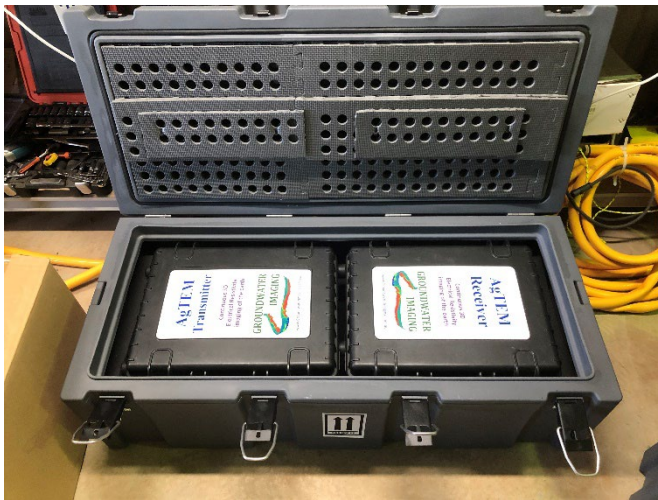
Figure 37 AgTEM electronics packaging. A test loop is beneath.
