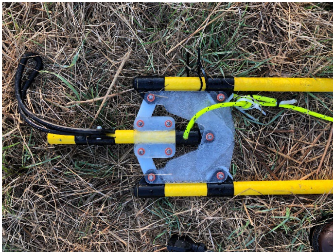
Figure 33 The Loop mounting end of the front loop booms.
