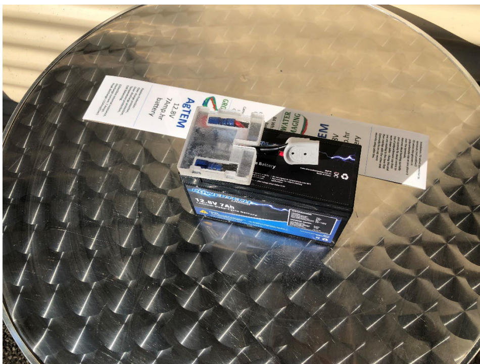
Figure 14 Slide connectors over terminals (red +, black -) and bend wires to fit in the protective cap. Then follow instructions on the decal to wrap all these parts. While the cap covers the terminal tabs, the tabs themselves prevent the cap from sliding out of position.
