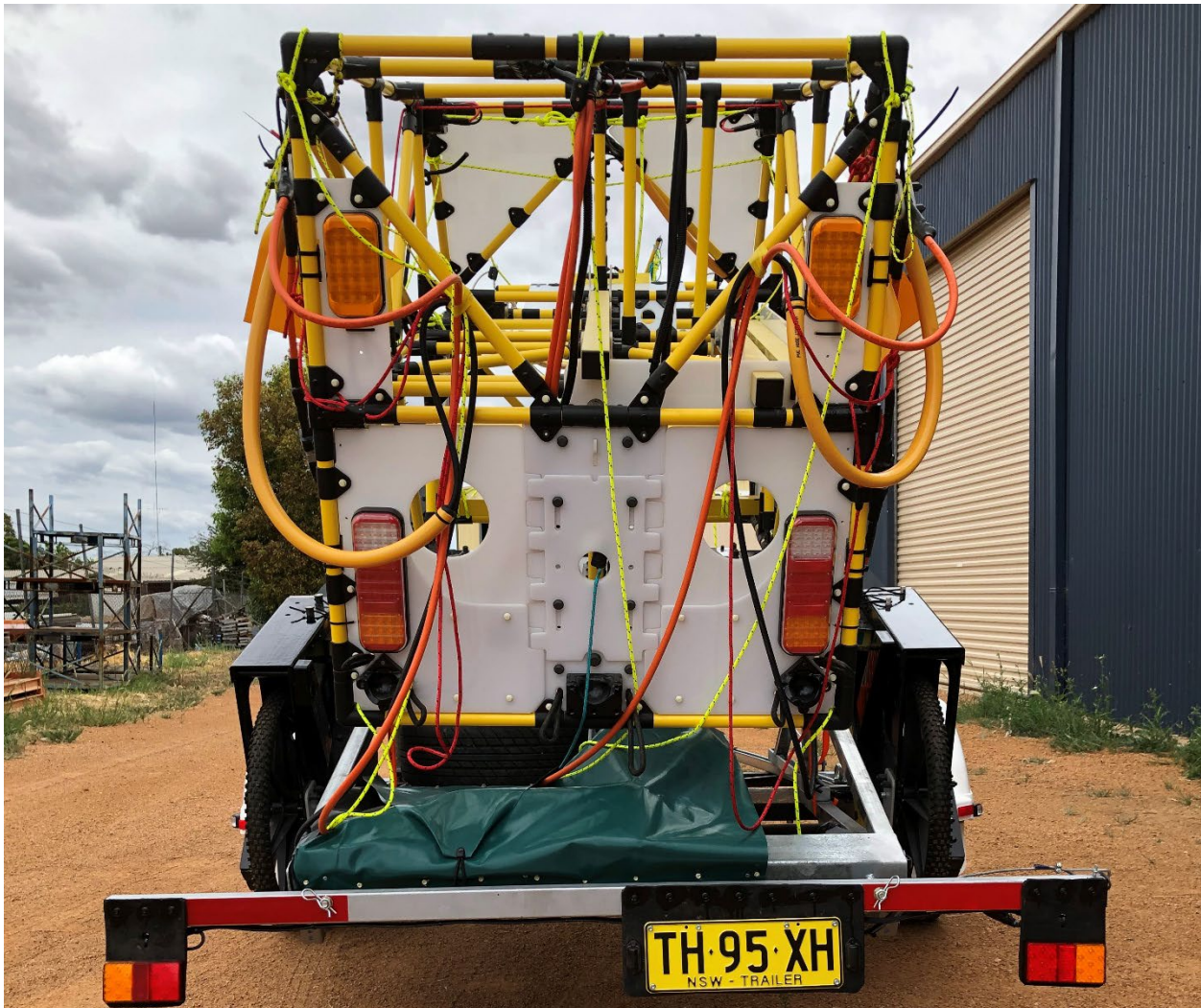
Figure 133 AgTEM-Wallaby secured on the float trailer, with tailgate reattached behind. Rigging is packed in the bag and rear booms slide, with rigging still attached, down a long cylinder hidden by the bag. AgTEM slides up onto the trailer along skids.
