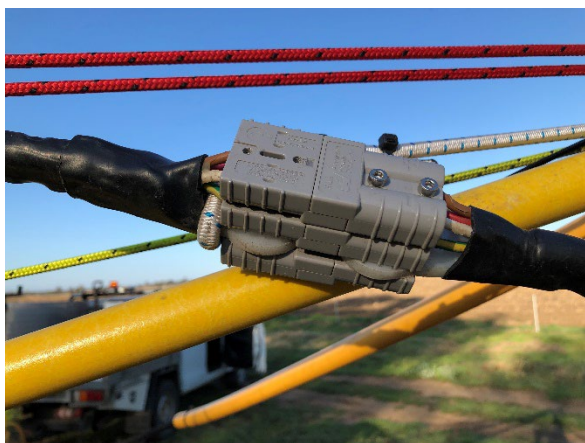
Figure 28 The transmitter loop is fixed to flying leads pulled elastically out each side of the Wallaby so that cable slack, needed for connecting the connector, is not near the Wallaby core where it would strongly affect mutual inductance nulling.
