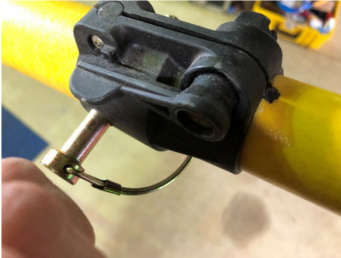
Figure 68 A recessed black dot aligns with the telescoping fixture seam to make re-aligning pins easy - booms should be extended to precise lengths for AgTEM requirements (including mutual inductance nulling) but generic ability to extend further exists.
