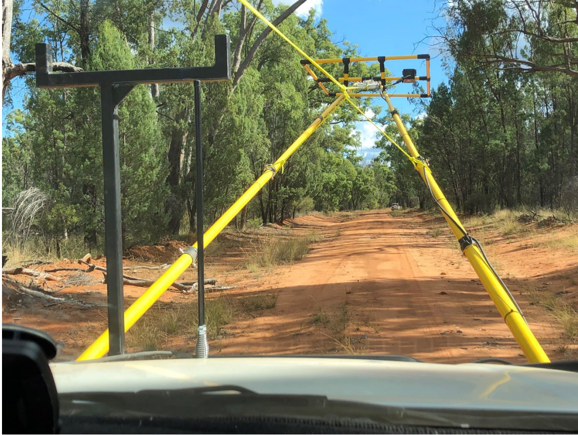
Figure 130 Front loop on suspended booms and gimbal mount. Area is 1.000 \times 1.600\text{m} \times \text{number of turns} \times \text{Pre-amp} . With 10 turns and 10.25x preamp this is 164
