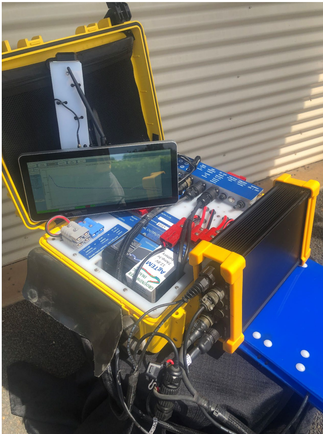
Figure 21 The new AgTEM electronics released by January 2025 has 3.3V to 18V variable loop power and air cooling internally so much of the old power management configuration is no longer required. An interim model in the USA in 2024 still with water cooling and in the old larger 6000 series case required adjustment of the variable voltage via a potentiometer. The new electronics is backpackable and one power supply can drive all parts due to extra filter circuits.
