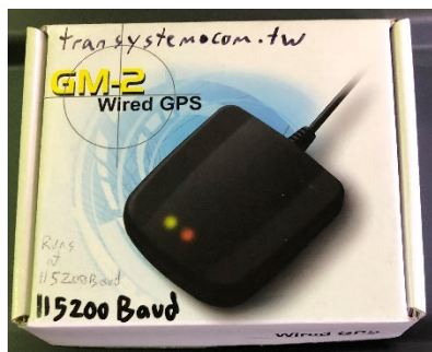
Figure 46 Low cost standard accuracy GPS from Transystem is all that is needed for Wallaroo survey positioning.
