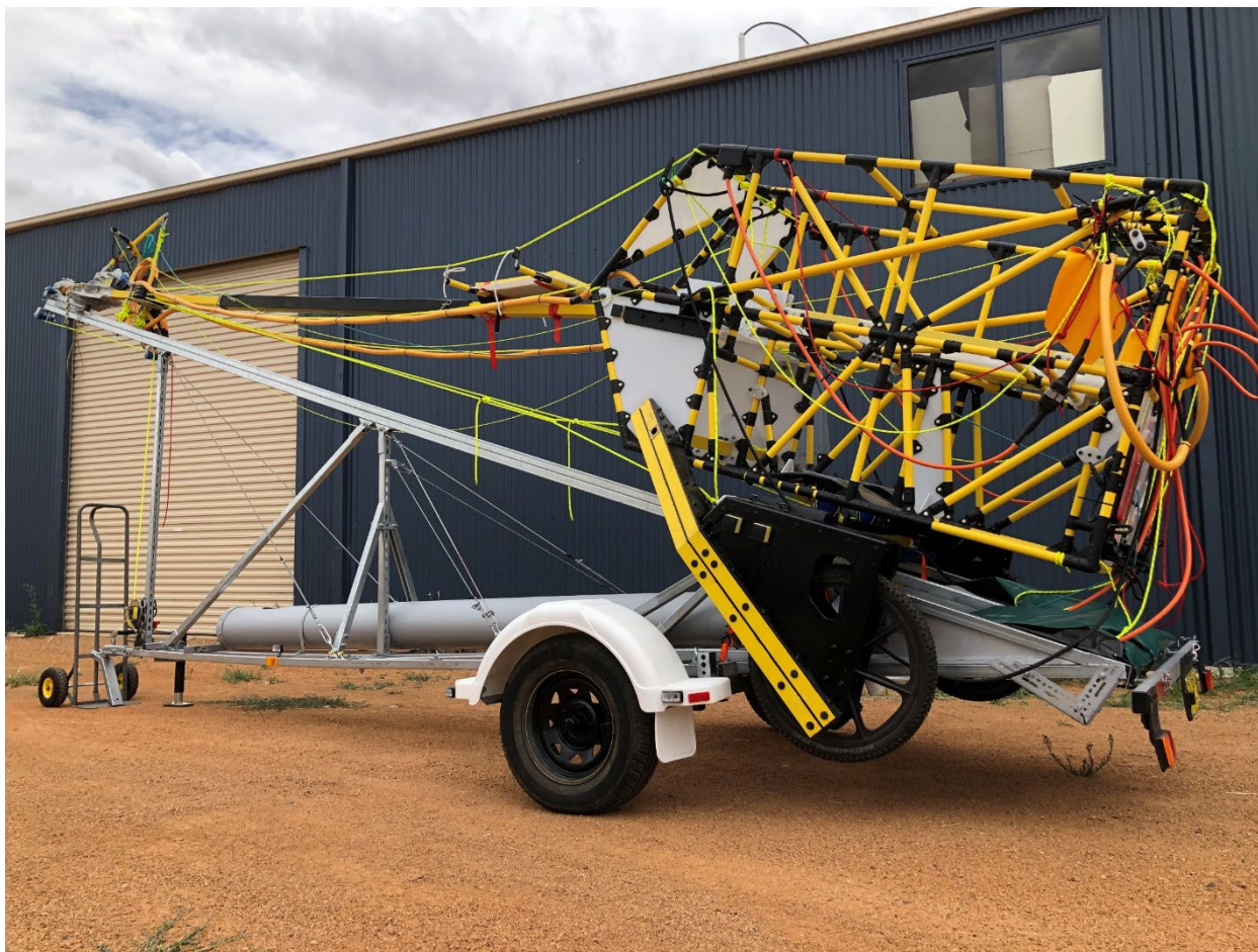
Figure 23 AgTEM stored on the quick deployment trailer
