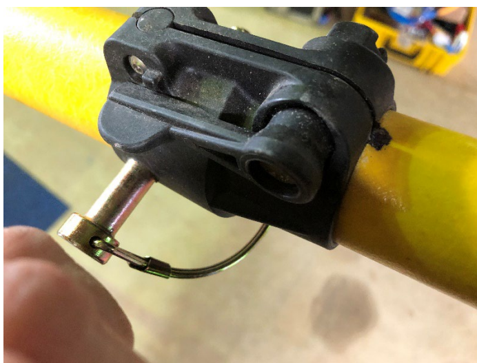
Figure 27 Small black indented marker dots align with clamp seams to indicate when boom extensions are aligned for inserting fixing pins.
