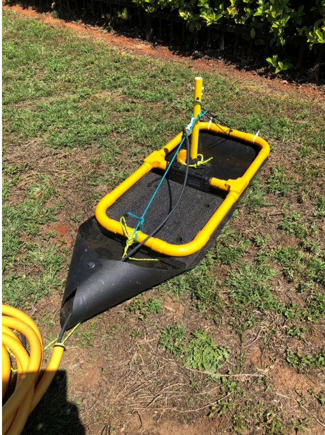
Figure 131 AgTEM-Wallaroo small towed receiver coil on a disposable mat. Foam distributes load to increase the life of the disposable sheet when dragged over gravel. The sheet is 1.6mm thick polyethylene.
