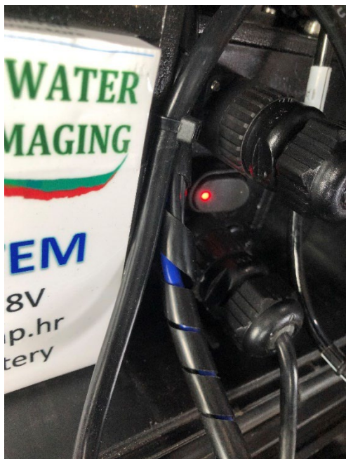
Figure 43 The receiver accessories case has power distribution incorporated. The On/off switch isolates all peripherals plus forced external ventilation. Connectors shown lead to batteries and to the computer power supply. More lead to the GPS display and receiver.
