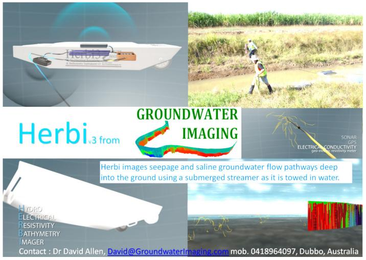
Investigation of seepage and saline inflow is our speciality. For this purpose Groundwater Imaging Pty. Ltd. supply a compact device for use on water which they call Herbi3 (Hydrographic Electrical Resistivity & Bathymetry Instrument). It is towed by walkers or behind a boat. A submerged streamer of electrodes senses multiple depths into the substrate with extra focus on the top decimetres where silt layers & clay lining need to be investigated.
