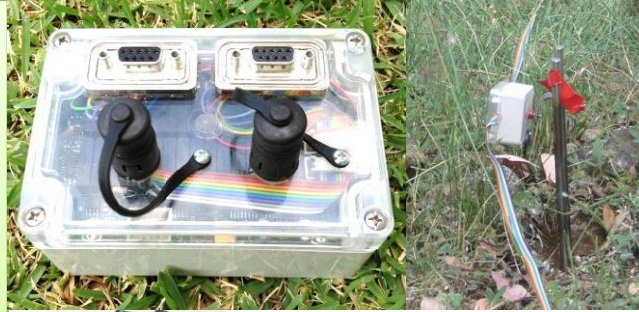
L-GM Geo-resistivity meter, 1 and 16 electrode switchboxes & telemetry modem.
