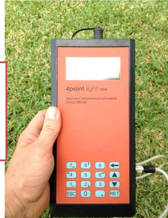
L-GM Geo-resistivity meter, 1 and 16 electrode switchboxes & telemetry modem.
